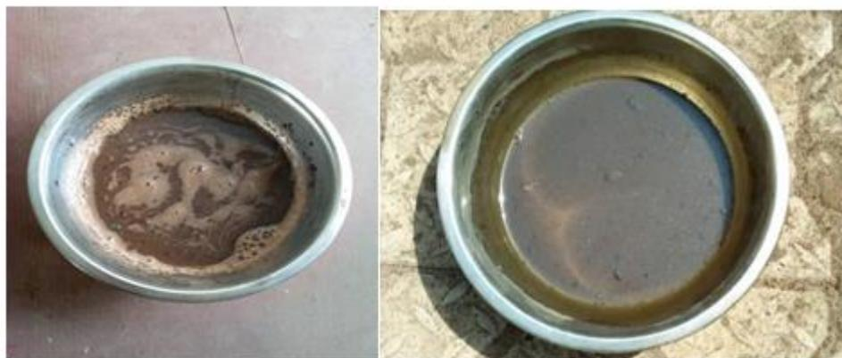
Fig. 1. Oil sheen test result for unpolluted soil (left) and crude oil polluted soil (right)
