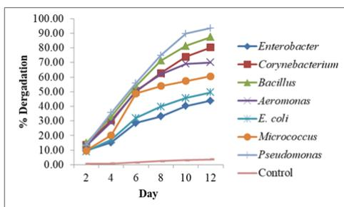
Fig. 4. Crude oil degrading potential of bacterial isolates in liquid medium
