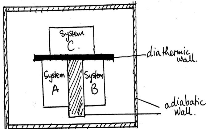
**Fig. 1: Bodies A and B are in Thermal Equilibrium with body C.**
