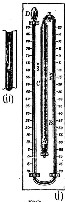
**Fig. 5: Maximum and Minimum (Six's) Thermometer**
