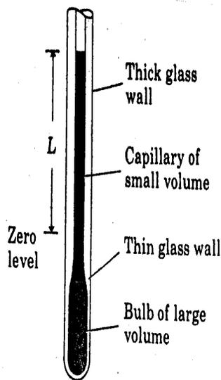
The liquid-in-glass thermometer makes use of either mercury alcohol. The laboratory thermometer, clinical thermometer and the Maximum and Minimum (six's) thermometer are the commonly used mercury-in-glass thermometers. However, the alcohol-in-glass thermometers are used in temperate countries because alcohol has a much lower melting point than mercury.
